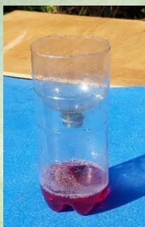
4. On the side of the bottle draw a scale in millimetres. You can draw this straight on to the bottle or on a piece of tape then stick it on.
